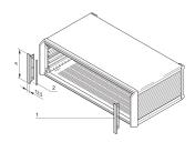
This kit can be used for covering the front frame and additionally shielding between the side panel and front panels.
