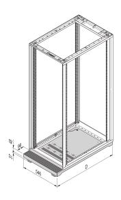
Aluminum mobile base plinth with load capacity of 200 kg, for aluminum cabinets with 600 mm breadth.
