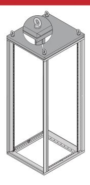
bolt on lifting eyes to lift and place cabinet without cabinet damage.
