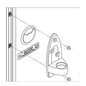
Mounting material to mount adjustible monitor arm at the cabinet exterior.
