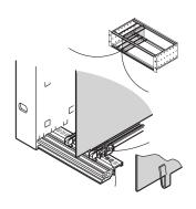
The divider plate enables the user to create a separate area inside a subrack or case. The plate can be clipped into the perforation of the horizontal rails. The subracks or cases have to be disassembled if the plate will be assembled.
