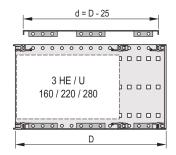
A cover plate is used for electromagnetic shielding or as mechanical protection. The cover can be screwed onto the side panel.
