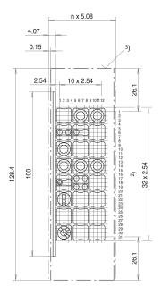
Mounting frame for mounting plane 1, Flammability UL 94 VO and two threaded female connectros M2.5.
