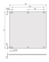
Front panel, unshielded, front anodized and rear conductive.
