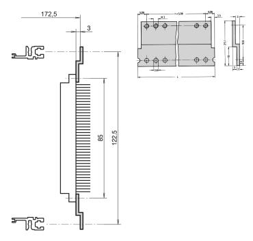
Z-rail for connector in accordance with DIN 41617, 31-pin.
