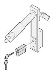
Profile cylinder is the most common form of the security door locks used today and a form of the locking cylinder. Semi-profile cylinders are generally flush with respect to the door and are easy to integrate into locking systems.
