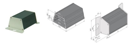
The Trapezoid Alu-profile case enables a user to insert 3 non standard PCBs. The PCBs will be inserted in grooves in the Alu-profile tube. Both sides are covered with 2.5 mm thick L-shaped front panels for wall mounting.
