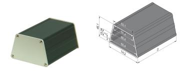
The Trapezoid Alu-profile case enables a user to insert 3 non standard PCBs. The PCBs will be inserted in grooves in the Alu-profile tube. Both sides are covered with 2.5 mm thick.
