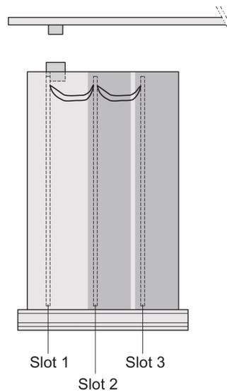
Frame type plug-in unit, non-shielded, perforated top / bottom cover, rear panel with cutout for one connector.
