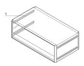
For EMC shielding between side panel and cover plate. The stainless steel shielding assembles to the cover and makes contact with the side panels.
