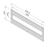
Front panel with cut-out in accordance with DIN 43880 (for power distribution modules).
