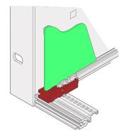
The PCB handle enables a user to extract a PCB without a front panel.
