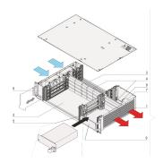
VME64x system for 4 horizontally mounted VME64x boards 6 U, 160 mm. Rear I/ O option. The power for the system is supplied by up to two pluggable power supplies. A hot swap fan tray with 4 fans guarantee an excellent cooling.
