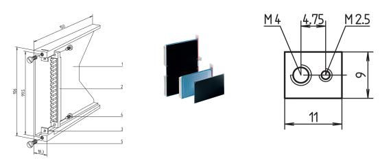
Accepts PCBs in Euroboard format, 100 x 160 mm. Plastic material PBT.
