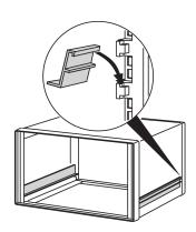
Slide rails are made from Aluminum profile, suitable as supports for 19" subracks and 19" chassis.
