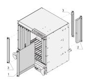
Advanced TCA front panels cover empty slots in a system. The additional air baffle blocks and guide the air in the right direction.
