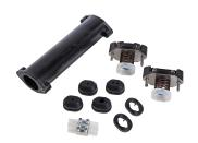
nVent RAYCHEM CS -150-UNI-PI is a universal underinsulation cold applied connection kit for polymer insulated (PI) heating cables, for splicing and connection of PI heating cables to cold leads (max 32A) or 3-core flexible power cableS (max 25A) using screw terminals. Approved for use in hazardous areas.
