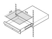
Writing surface to use with our 19" drawer. It is placed on the drawer and can be lifted up when the drawer is open.
