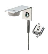
The nVent CADDY Speed Link Light Pack with Nail Gun Bracket includes a precut length (1m and 2m) of 1mm wire rope riveted to an angle bracket designed for direct fastening together with an ultra-low-profile locking device. Contractors can quickly and safely install it to the concrete ceiling using a wide range of nail guns to support and secure lighting and signage.
