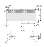
The perforated rear panel, Al, 2.5 mm is unshielded. The rear side is conductive.
