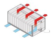
The Self-adhesive seal closes the space between the rear horizontal rail and base plate to avoid an air short cut in RatiopacPRO Air case.
