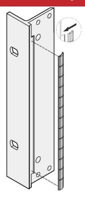
The stainless EMC gaskets are inserted into a slot on the right hand side of the U-shaped front panels.
