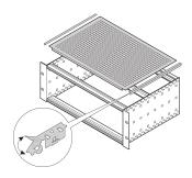
A cover plate is used for electromagnetic shielding or as mechanical protection. The cover can be used is non-standard boards will be assembled into the subrack.
