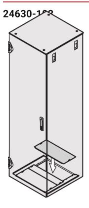
Cover Plate for Base Plate helps cover the base plate openings which could have been otherwise used for cable management.
