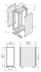
The nVent SCHROFF RatiopacPRO tower case provides electronics protection for 19" assemblies. This flexible and robust case is simple to convert from desktop to a 19" rack mount case and includes four different style options. This version of the case provides a sleek design and feet for desktop applications.
