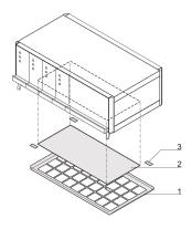
The air filters the intake air and reduces the quantity of dust or other particles.
