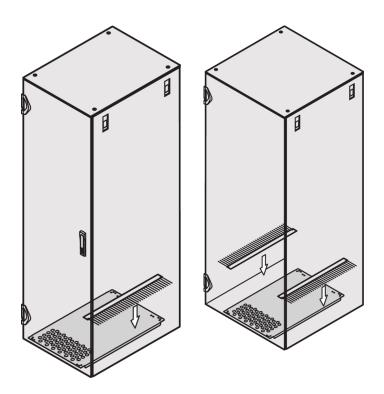
Multi Piece Brush strip to close side opening of base plate (for side cable routing); 1 brush strip for various breadths.
