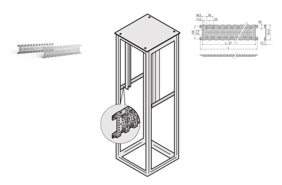
Horizontal depth member in the cabinet depth. Mounted directly at the Varistar CP frame for cable management, increased frame stiffness and additional fixing points.
