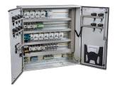
nVent RAYCHEM SBS-XX-SNR control panel provides an integrated solution for nVent RAYCHEM self-regulating heating cables in sprinkler freeze protection applications. It offers multi-circuit, multi-sensor and multi-control with integrated electrical protection, with redundant circuit automatic switching capability compliant with BS EN 12845:2008. A 400 VAC (3 phase) supply is required.
