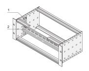
Support rail to clip on retainer of modules in accordance with DIN 43880 like fuses or circuit breakers.
