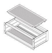
A cover plate is used for electromagnetic shielding or as mechanical protection. The cover can be screwed onto the side panel.
