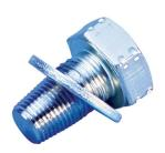
The ELFB taper bolt is used to firmly attach a nVent LENTON taper-threaded coupler onto formwork in precast and cast-in-place construction. This reusable form saving accessory allows forms to be pre-drilled with the correct spacing of the reinforcing steel, which speeds construction and allows the forms to be re-used on repetitive construction elements. This system can be used in conjunction with coupler boxes to eliminate the use of bend-out-boxes and also helps eliminate protruding dowel bars.
