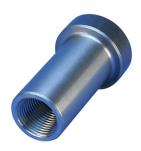
One-piece flange couplers are ideal for eliminating protruding dowel bars in segmental pour applications. The flange side of the coupler is typically tack or seal welded to cast-in-place structural steel walls commonly found in most modern nuclear reactor designs.
