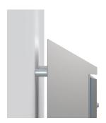
Mounting brackets for hygienic wall fixing. Provides an space between the enclosure and the wall to facilitate cleaning operations. It includes the sealing washers to guarantee the IP rating. Machining required. Design according to EHEDG standards.
