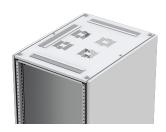
Up to four ventilation fans can be mounted on this roof plate, which means that the enclosure can be cooled in incremental steps, depending on the number of fans fitted. Brushes fitted to the cable openings allow for different cable diameters to be installed easily.
