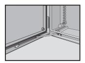
Door Stop Kit limits door to 120-degree opening. Field installable on all sizes of Ultrx enclosures.
