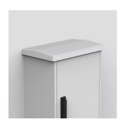
A polyester rain hood provides shelter via a sloped roof and protects installed components from accumulated water dripping into the enclosure when the door is opened.
