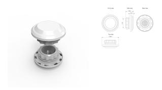
The pressure compensation plug equalises the pressure that occurs, due to temperature differences, inside the enclosure with the outside environment, while reducing the risk of dust entering the enclosure.
