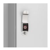
The padlocking cover is mounted over the existing standard lock. The standard lock is totally covered and not accessible when padlock is fitted. Maximum padlock bow diameter of 10 mm.
