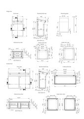
The stainless steel compact console, MPGS, in a IP66/55 protection degree is available off the shelf. It has a hinged desk panel, and the ergonomic design allows for easy installation and access to HMI-equipment- It also increases the mounting space available. This console can be installed in virtually any environment, grade dependent.
