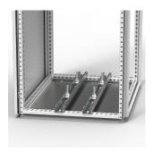
This heavy duty carrier bar for mounting heavy components, such as transformers, is supplied with T-shaped sliding bolts and is equipped with slotted holes for mounting in any position within the enclosure.
