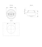
This two component cable gland can be mounted on a wide range of enclosures. It secures the cable into position, and eliminates any external strains.
