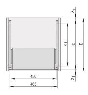
Telescopic slides with guiding profile for fitting in cabinets with 25 kg load capacity.
