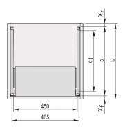
The C-profile, assembled on the Side Panel of the subrack serves fixes the subrack on the guiding profile when mounted into a cabinet.
