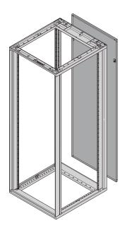
Steel Rear Panel for aluminum extruded enclosure is connected with 2 twist-locking catches (Torx T30, with 1/4 turn).
