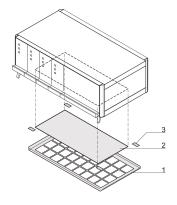
The replacement air filter Kit can be replaced if the original air filter is dirty to optimize the air flow into the case.
